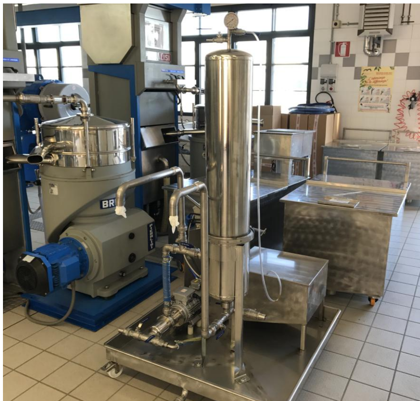
Figure 116: vertical separator and column filter
