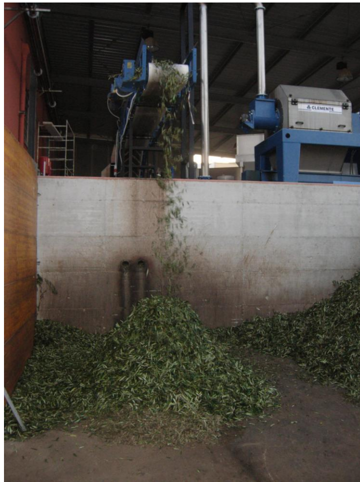
Figure 135: leaves resulting from the cleaning of olives in the mill
