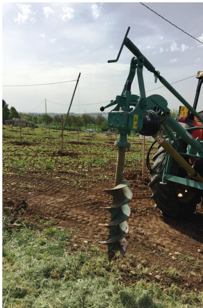
Figure 24: auger for making holes
