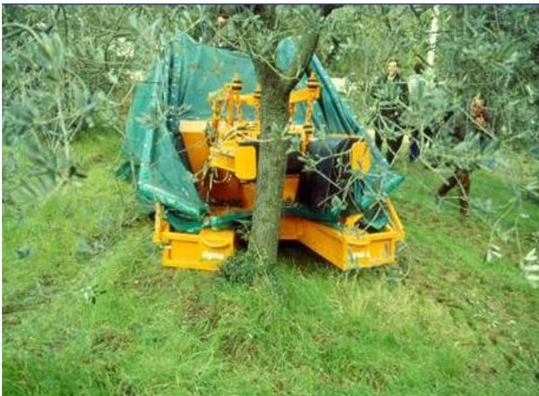
Figure 106: for the application of the shaker the trunk must be at least one meter high and the main branches in the vase must be raised
