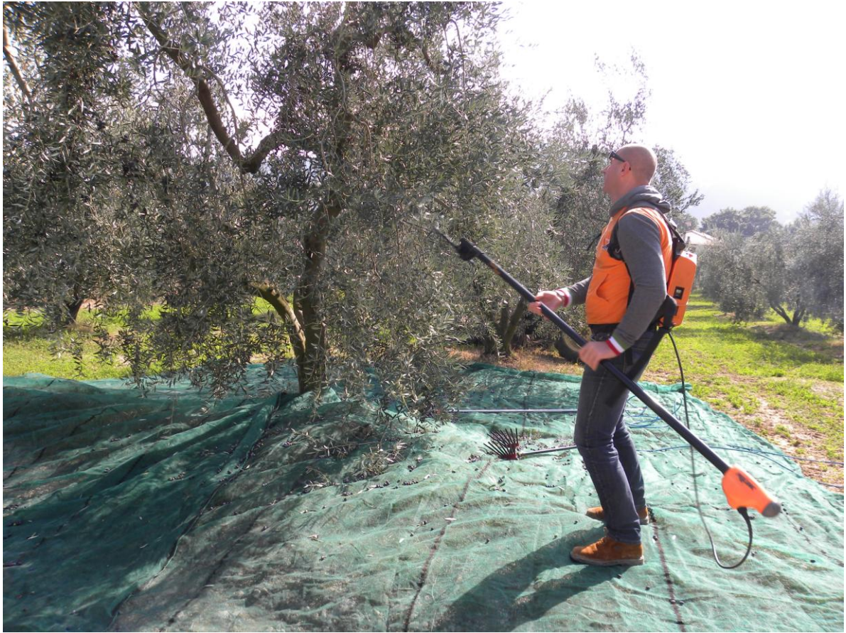
Figure 102: harvesting with electric comb
