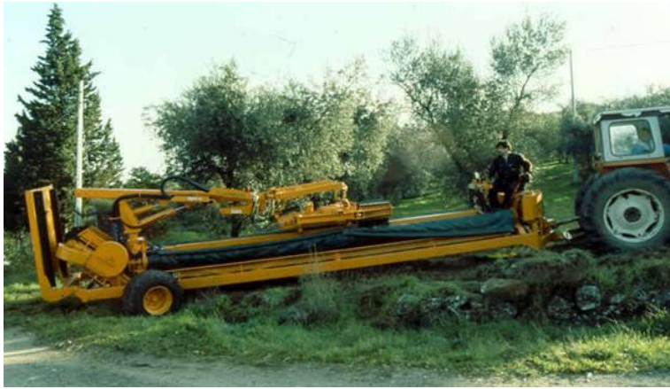
Figure 109: trunk shaker with trailed interceptor frame
