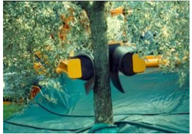
Figure 109: trunk shaker with trailed interceptor frame
