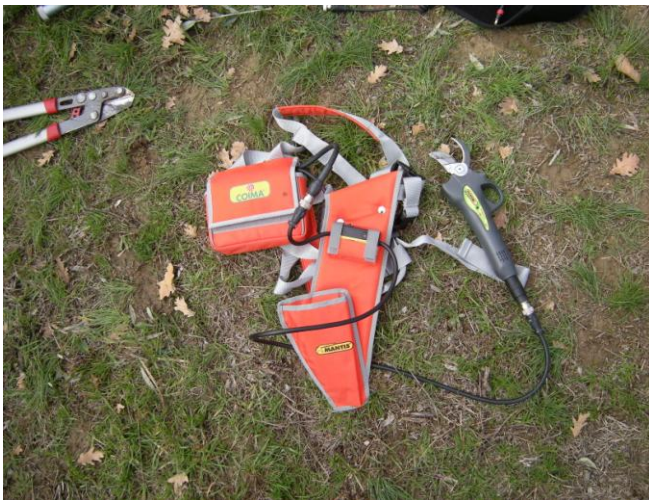
Figure 88: electronic scissors with battery
