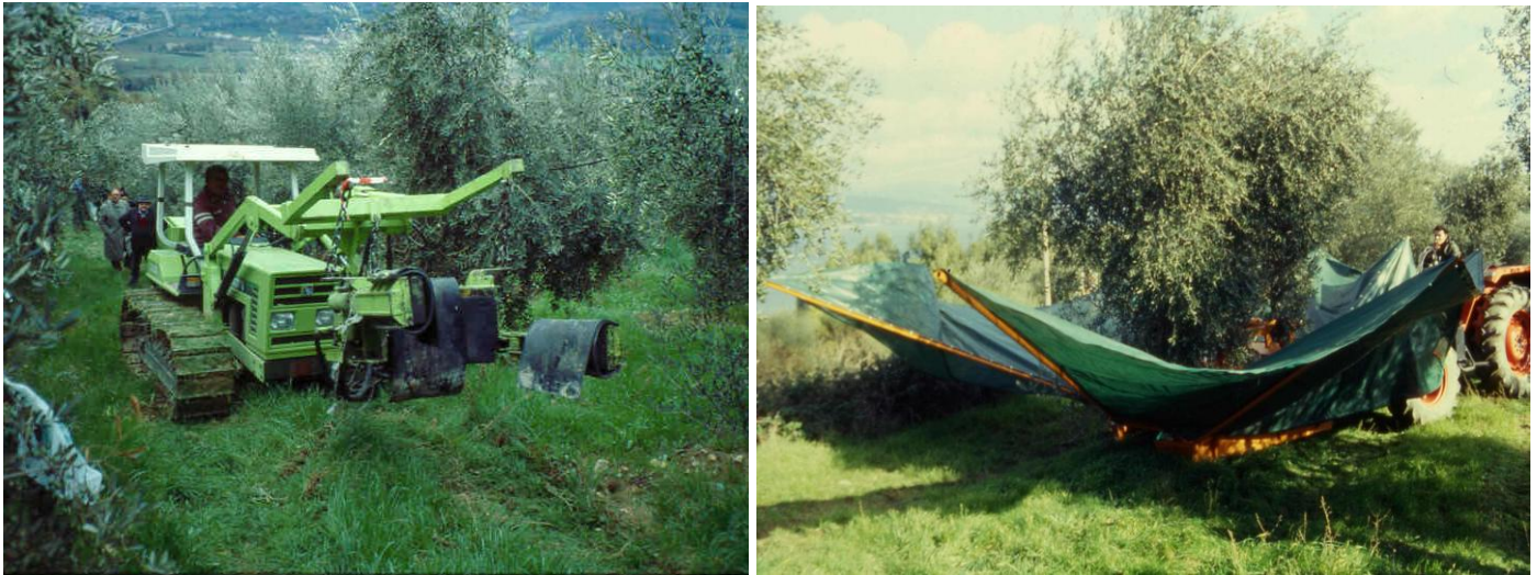
Figure 105: shaker without and with interceptor frame
