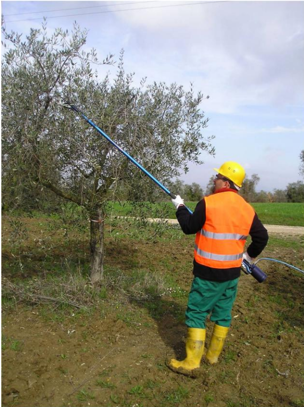
Figure 87: operator using a pneumatic shear mounted on a rod and wearing personal protective equipment
