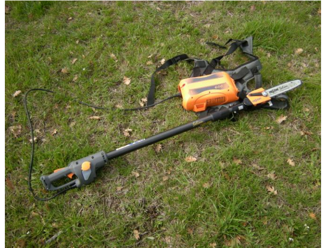
Figure 89: electronic chainsaw mounted on a telescopic pole with a battery carried by a vest
