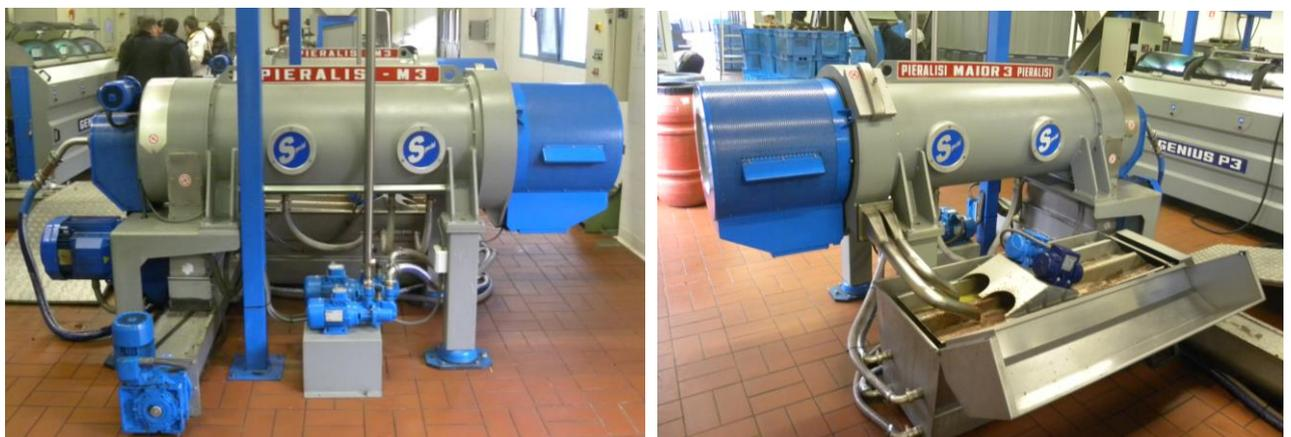
*Figure 115: centrifugal extractor*
