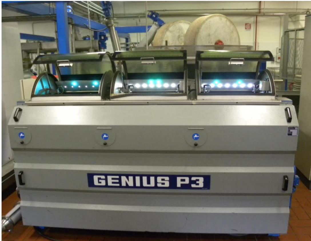
**Figure 114: crushing and kneading machine**
