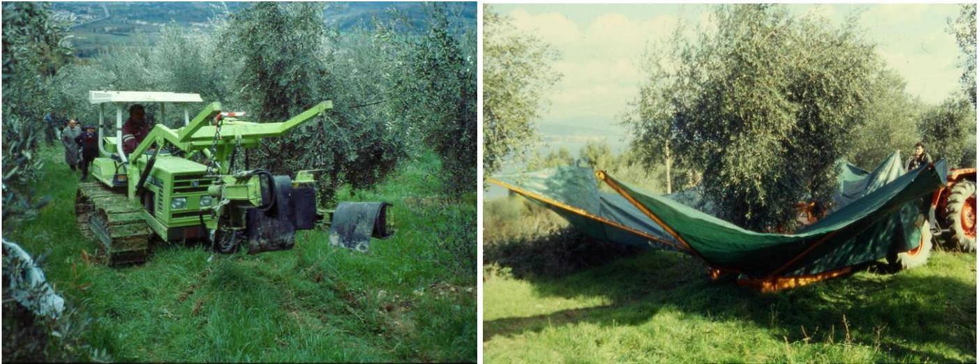
**Figure 105: shaker without and with interceptor frame**
