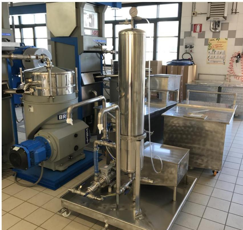
**Figure 116: vertical separator and column filter**
