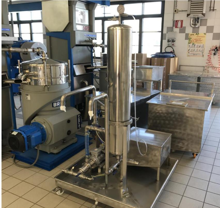
**Figure 116: vertical separator and column filter**
