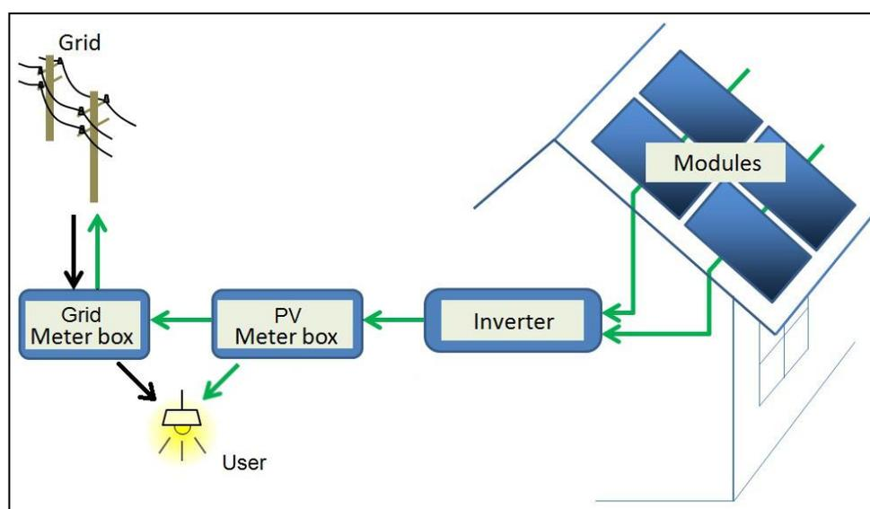
*Figure 126: main components of a PV system*
