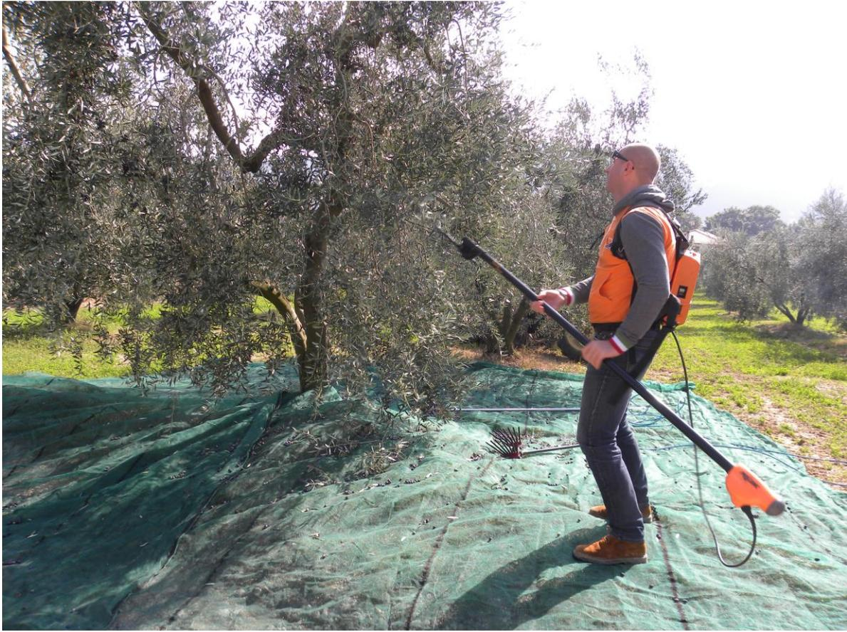
**Figure 102: harvesting with electric comb**
