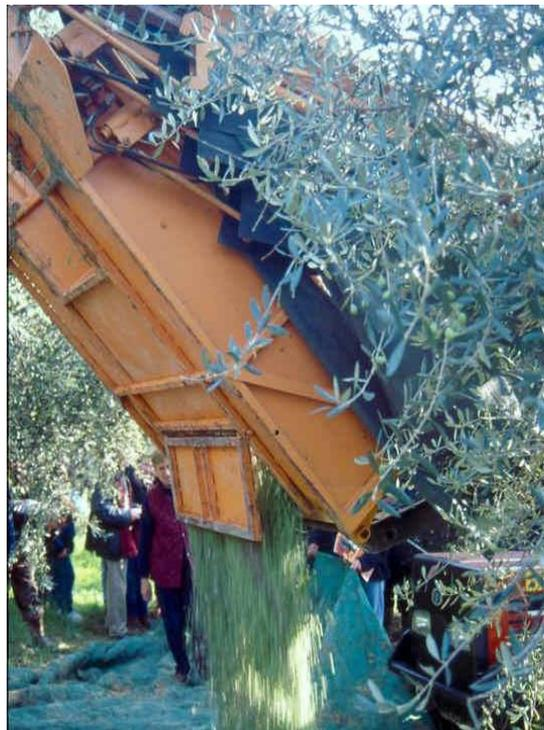
***Figure 108: unloading the olives harvested with a shake***
