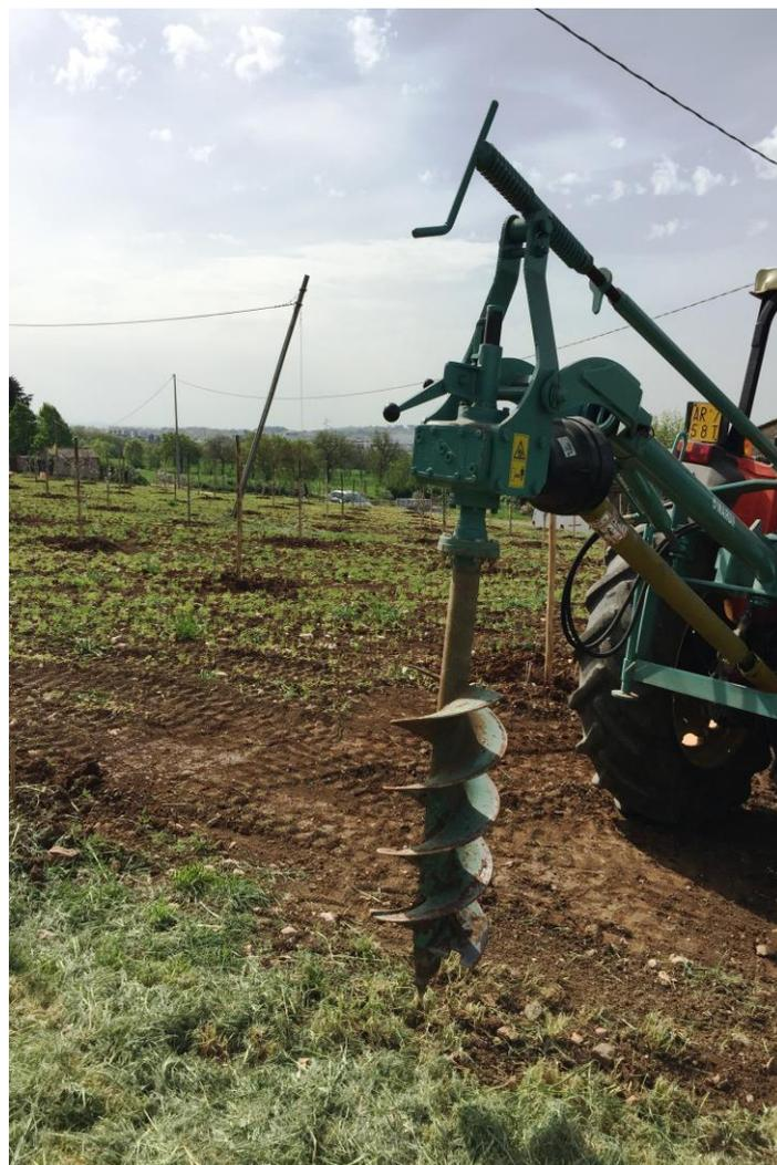
**Figure 24: auger for making holes**
