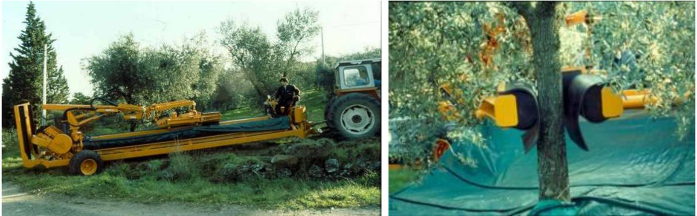
**Figure 109: trunk shaker with trailed interceptor frame**
