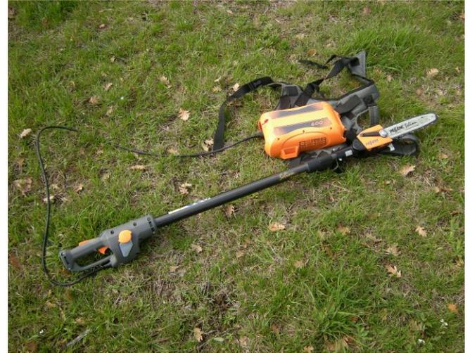
**Figure 89: electronic chainsaw mounted on a telescopic pole with a battery carried by a vest**
